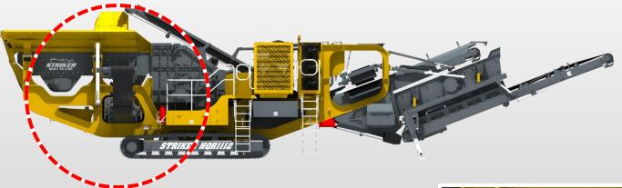
By-Pass chute removes natural fines from the feed material and discharge onto the "Side Discharge Conveyor"
