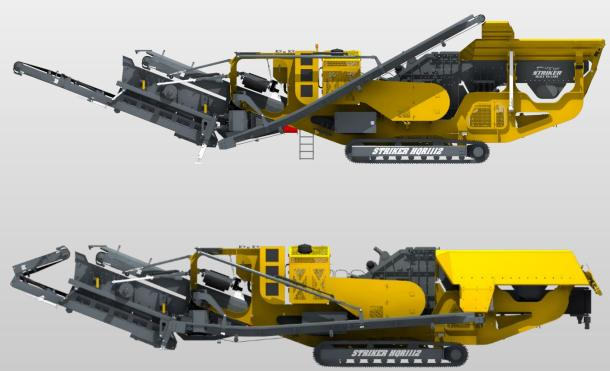
**NOTE:** Higher & Wider – Track width increases 400mm and raises 200mm. This gives increase ground clearance and maintenance access.
