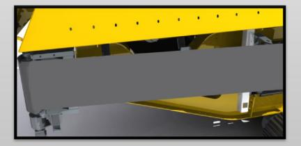
The by pass chute transfers removal of fines on to the side discharge conveyor
