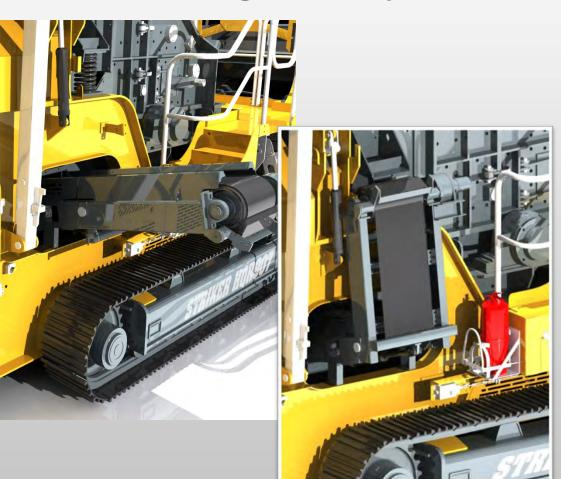
Hydraulically folding side discharge conveyor
