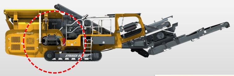
By-Pass chute removes natural fines from the feed material and discharge onto the "Side Discharge Conveyor"
