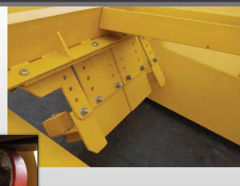
Hydraulically lifts up into the operating position raising the feeder on rollers under the feeder belt
