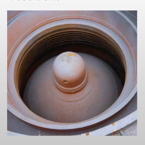
Bowl is designed to spread the feed material equally around the cone opening
