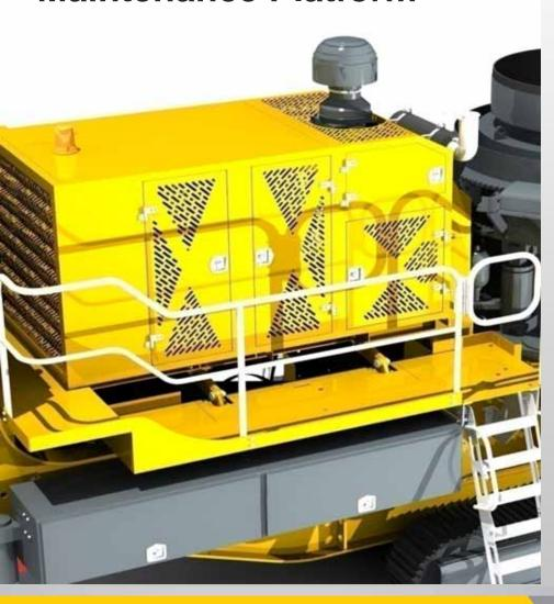
All round access platforms for maintenance on the diesel engine
