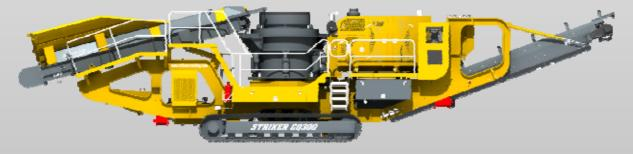
**NOTE:** Higher & Wider – Track width increases 400mm and raises 200mm. This gives increase ground clearance and maintenance access.
