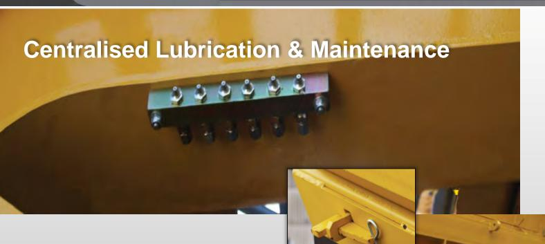
Centralised braided greasing lines for feed conveyor bearings and product conveyor
