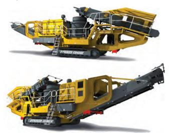
**Belt Feeder** - Feeding the material into the Cone Crusher is a belt feeder. Contained under the loading area are impact rollers for loading shock absorption while the heavy-duty feeder belt feeds the cone via a hydraulic variable speed drive motor. Fitted into the conveyor is a metal detector to protect the cone from tramp metal.
