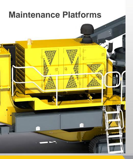
All round access platforms for maintenance on the diesel engine
