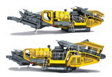
**Belt Feeder -** Feeding the material into the Cone Crusher is a belt feeder. Contained under the loading area are impact rollers for loading shock absorption while the heavy-duty feeder belt feeds the cone via a hydraulic variable speed drive motor. Fitted into the conveyor is a metal detector to protect the cone from tramp metal.
