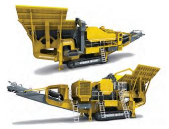
Vibrating Grizzly Feeder - Feeding the material into the Jaw Crusher and/or fines chute is a vibrating grizzly feeder including :
