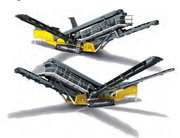
**Main Chassis -** Main chassis members are constructed from welded beams. These members are engineered to withstand the stresses exerted upon them by both road transport and operation of the plant.
