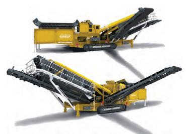
**Main Chassis -** Main chassis members are constructed from welded beams. These members are engineered to withstand the stresses exerted upon them by both road transport and operation of the plant. The chassis supports all the individual items of the plant and has integral onboard hydraulic stabilising systems for ease of setup on site.
