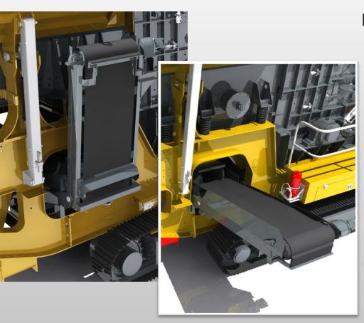
Hydraulically folding side discharge conveyor
